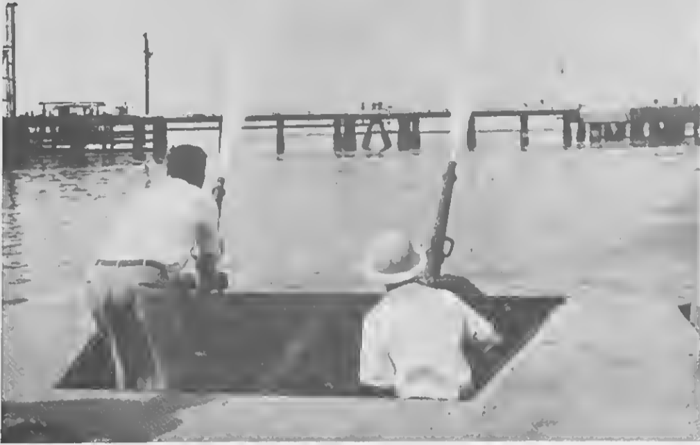
THE RANGE of the two turret nozzles on the Marine Department's new No. 9 fire boat is a healthy 75 feet with salt water and over 50 feet with foam. A pressure of 100 pounds is delivered by the boat's fire pump engine which was salvaged from an old launch and rebuilt by Mechanical Department personnel.
